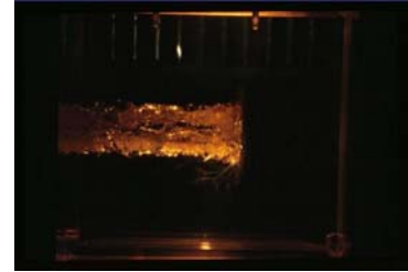
Figure 3: Plastic block damaged by a very high dose of proton radiation. The beam entered from the left. The precise radiation falloff at the end of range can be seen within the block
