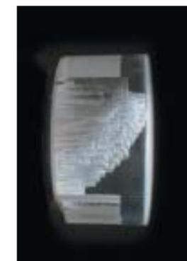
*A Lucite compensator is custom milled and shaped to the depth profile of the lesion for each beam used. The compensator is attached to the front face of the aperture. The Lucite controls the penetration of the protons, which go through the aperture opening. At any point within the compensator the thickness of the Lucite will proportionally reduce the depth of the protons passing through the device. The diagram shows the direction of the protons incident on a compensator.*
